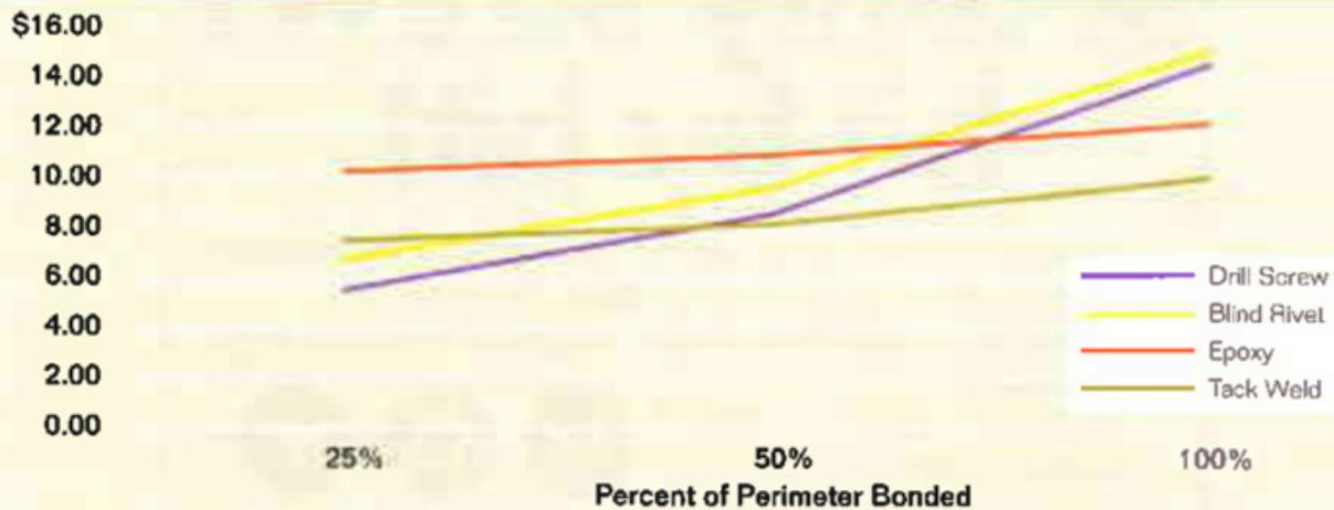
**FIGURE 2. Cost for Equivalent Shear Strength – 50% Bonded**
